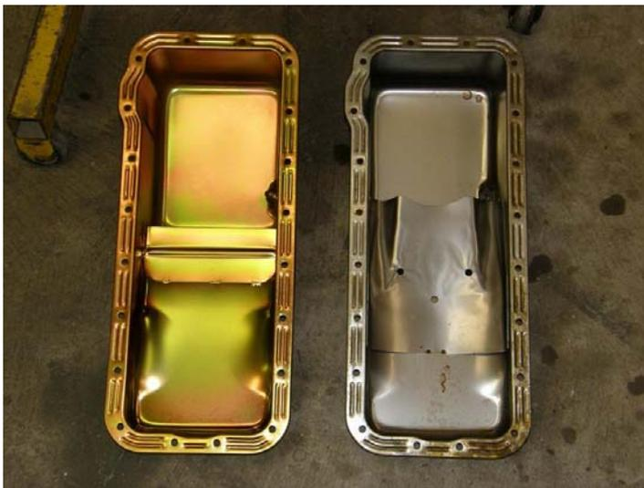
The factory oil pan shown on the right is not ideal for performance use. The baffle contacts the bottom of the pan near the back of the engine, and there are open spaces at the contact point allowing oil to pass under. On acceleration the oil can race away from the pickup causing oil starvation. The Milodon pan is superior due to the tight fitting baffle positioned farther forward in the pan, and should be considered a minimum for any serious performance use.
