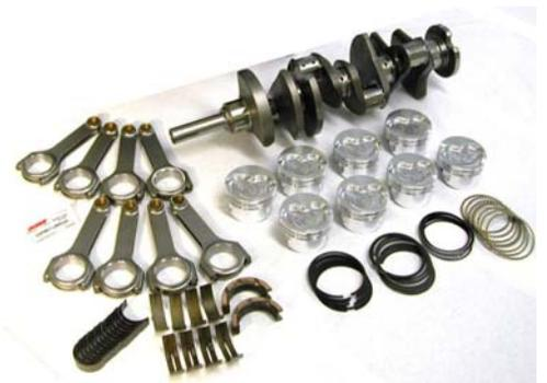
Survival Motorsport’s basic stroker kits include a cast Scat crank, 6.700” I-beam rods, and Probe pistons, plus rings, bearings, and balancing. The deluxe kit upgrades to H-beam rods and Diamond pistons, plus a better bearing package. The basic kit is suitable for most street applications, while the deluxe kit is just right for track use.
