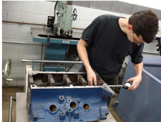
Bryan Hansen at R&R Performance measures the diameter and runout of the 390 block's main bearing bores. A straight machinist's bar was laid into the main saddle, and feeler gauges were used to see if any of the main bearing bores were out of alignment. The bores proved straight, but a check of the roundness with the dial bore gauge showed the bores were slightly egg shaped, so the block was align honed.
