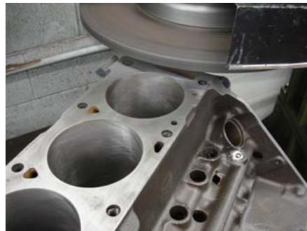
We needed to cut the decks a total of .022" on both sides to true them up. The plate bolted to the block was also used as a reference when setting up the machine used for this operation.
