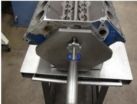
Next this plate is bolted to the block, indexing the crank centerline and the cam centerline. The 45 degree flats on the plate will be used as a reference to measure the block decks.
