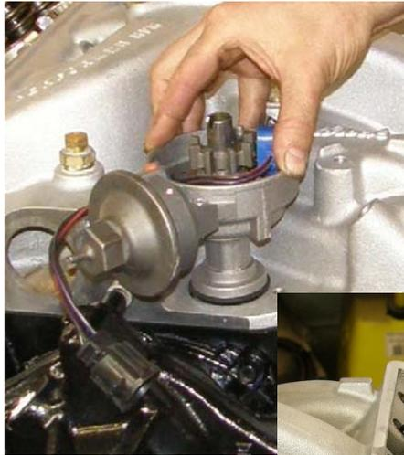
Installing the intake is a tricky part of FE engine assembly. After setting the intake down on the engine with the gaskets in place, temporarily install the distributor and move the intake fore and aft to get the distributor hole in the manifold. Now scribe a line across the valve cover rail on the intake and the head on each side, so that you can reinstall the intake again later and keep this alignment. If the distributor hole in the intake is misaligned with the distributor, it will leak oil.
